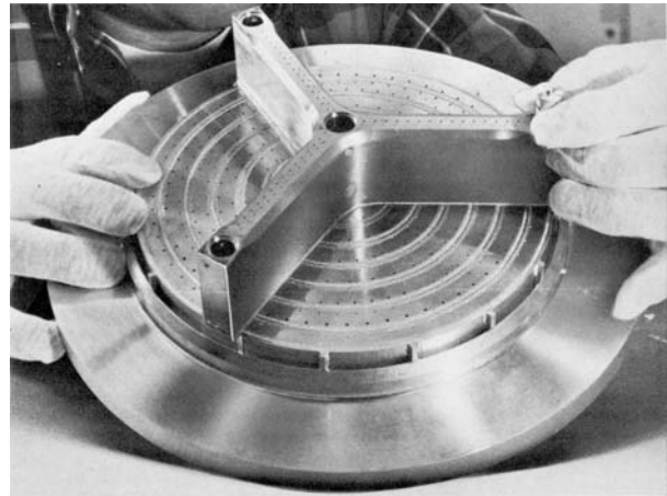
FIGURE 8.8. An injector with baffles and azimuthal slots (Harrje and Reardon 1972).
